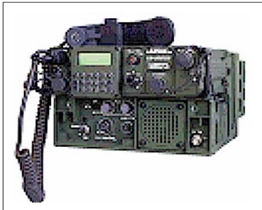
Figure I-1 Vehicular Mounted 20-Watt HF Radio System
